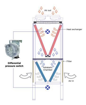
Differential pressure switch is an electro-mechanical device which is used for sensing a difference in pressure between two points.
